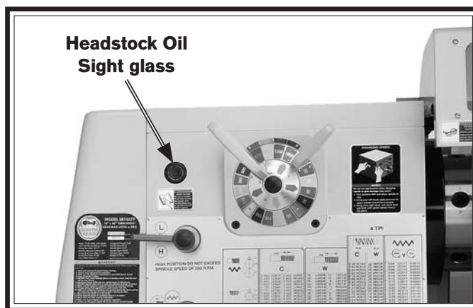
Figure 29. Headstock oil sight glass.
